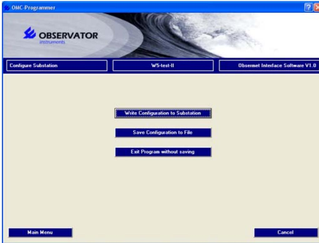
The choices in this screen are clear. The configuration can be written to a substation, the configuration can be saved to a file or you can exit the program without saving the configuration. Each follow-up screen has its own help-function.
