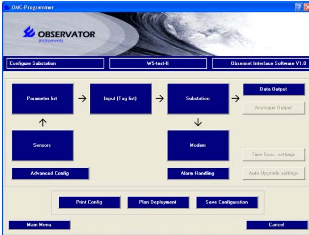
The total configuration of the substation is displayed on this overview.
