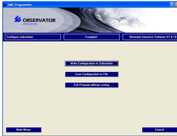
The next step is 'Write configuration to substation' to upload it in your OMC-045-III.
