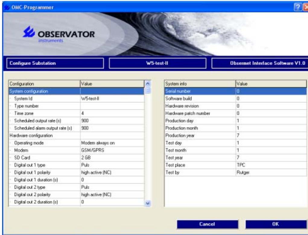
With this option you can change the advanced settings of the substation. It is also possible to configure additional hardware to add additional functionality to the substation. This means sending out e-mails and SMS a modem-board should be configured. For storing data it is necessary to configure a SD card.
