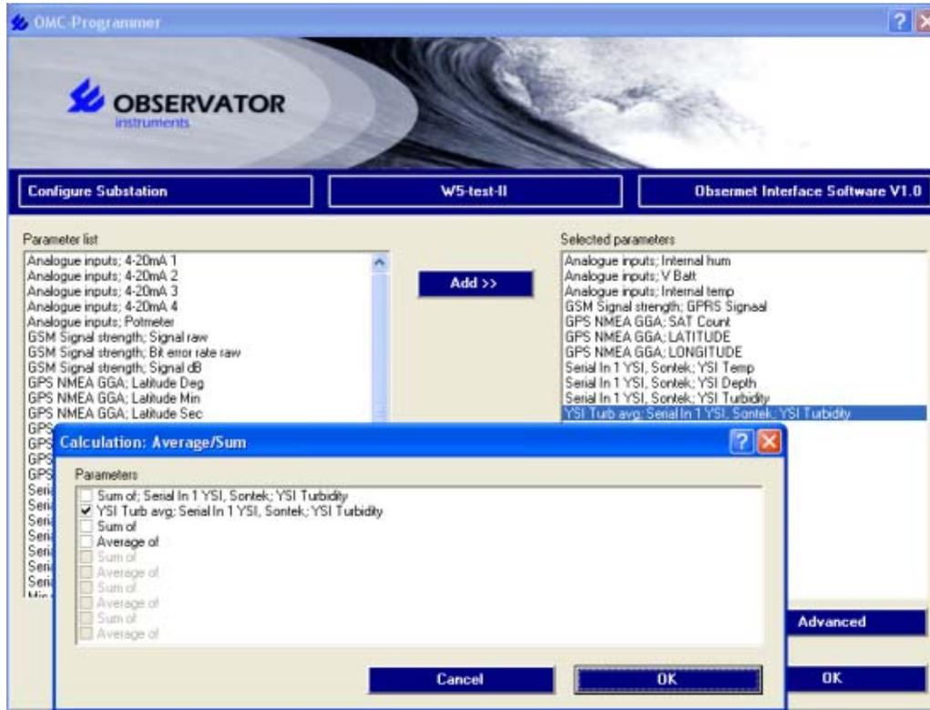
At this screen you can configure calculated parameters. A calculated parameter is a parameter which is the result of a mathematic calculation of a measured parameter. A calculated parameter will be calculated over the calculation rate.
