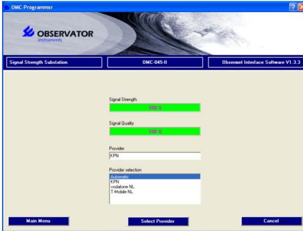
Using this option it is possible to check the GPRS signal strength & quality. Using this it is possible to point a antenna in the direction with the best GPRS signal. Before deployment it is very wise to check the signal strength & quality at the site first. A low signal will cause problems sending data.
