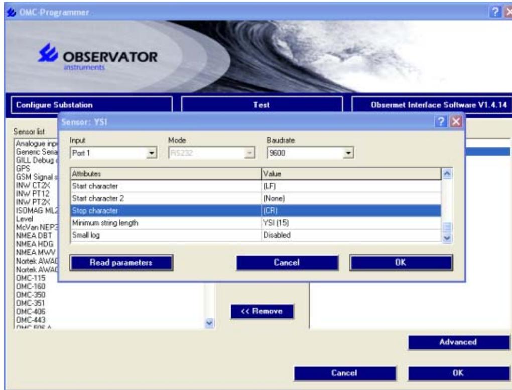
For the YSI the button 'Read Parameters' is included. This button will read the settings from the the YSI, so you won't have to set the parameters yourself.
